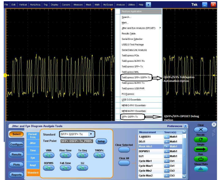
Tektronix SFP+ QSFP+ Tx - is developed on a Real Time Oscilloscope platform, which is the platform of choice for engineers designing their products around SFF-8431 & SFF-8634 technology. Option SFP-TX and SFP-WDP enable both an Automation Solution (for Compliance) and DPOJET Option (for Debug). Users can save up to 80% on testing time compared to manual testing. TWDPc - Transmitter Waveform Distortion Penalty for Copper Measurements are available with Option SFP-WDP. SFF-8431 SFP+ TWDPc based Matlab code is integrated into the SFP-WDP option to make sure Engineers can use this measurement in the automated setup.
